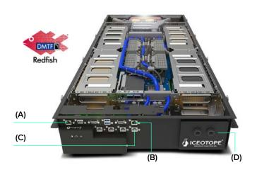
The server integrated in the Iceotope enclosure is connected to the IO ports on the front panel. Iceotope BMC (C) can be interrogated using a standard Redfish Compliant interface.
