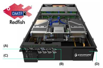
The server integrated in the Iceotope enclosure is connected to the IO ports on the front panel. Iceotope BMC (A) can be interrogated using a standard Redfish Compliant interface.
